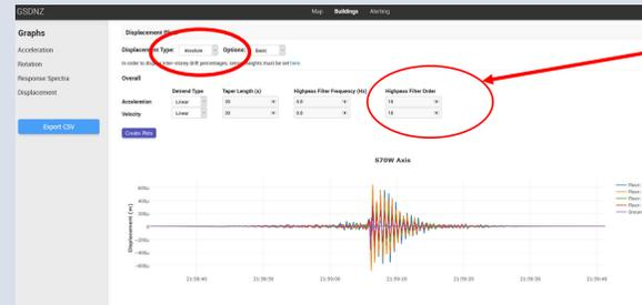
Change the high-pass filter frequency to 0.8 to remove noise.
