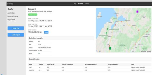
Shows the event, sensors that triggered, acceleration on north/south, east/west and vertical in G force.
