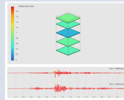
Floor of a building will change showing the vertical displacement recorded by the sensor, as the event trace runs
