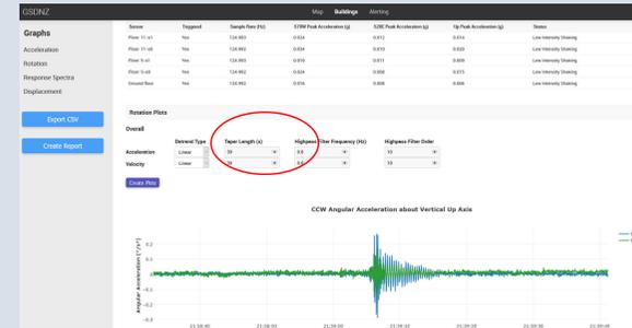
Rotation is calculated by placement of two sensors on a floor, then two sensors on a different floor with sensors in the same floor position. Change the high-pass filter frequency to 0.8 to remove noise.
